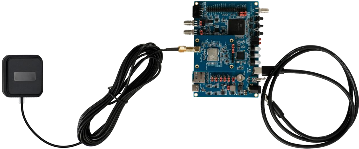
Figure 2: GNSS Module TE-A and Kit Components Mounted on EVB (Without 4G Module TE-A)
