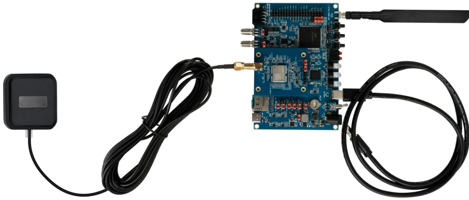
Figure 3: GNSS Module TE-A and Kit Components Mounted on EVB (Top View)
