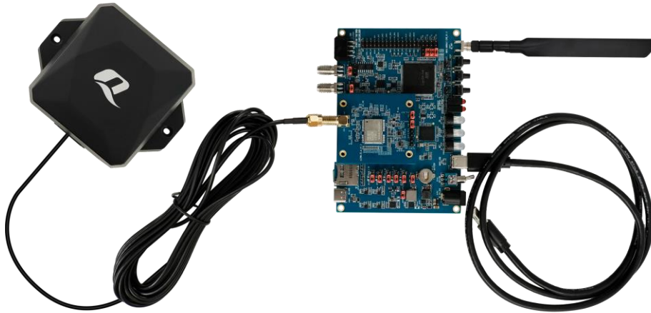
Figure 3: GNSS Module TE-A and Kit Components Mounted on EVB (Top View)
