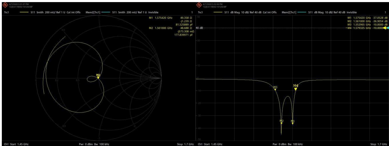
Figure 23: GPS + BeiDou Patch Antenna Test Result with Ground Plane of 100 mm × 60 mm
